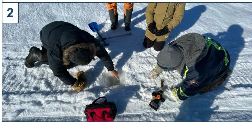
Snow and superimposed ice layers were identified and measured using snow pits. Snow density samples were collected at certain snow pits.
