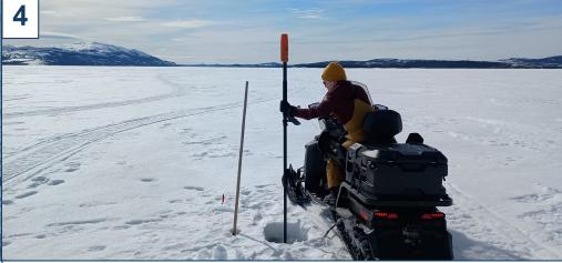
Point-based snow and ice measurements along the GPR transects were geolocated using a DGPS.
