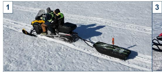
160 and 450 MHZ ground penetrating radar (GPR) surveys were conducted along marked transects.
