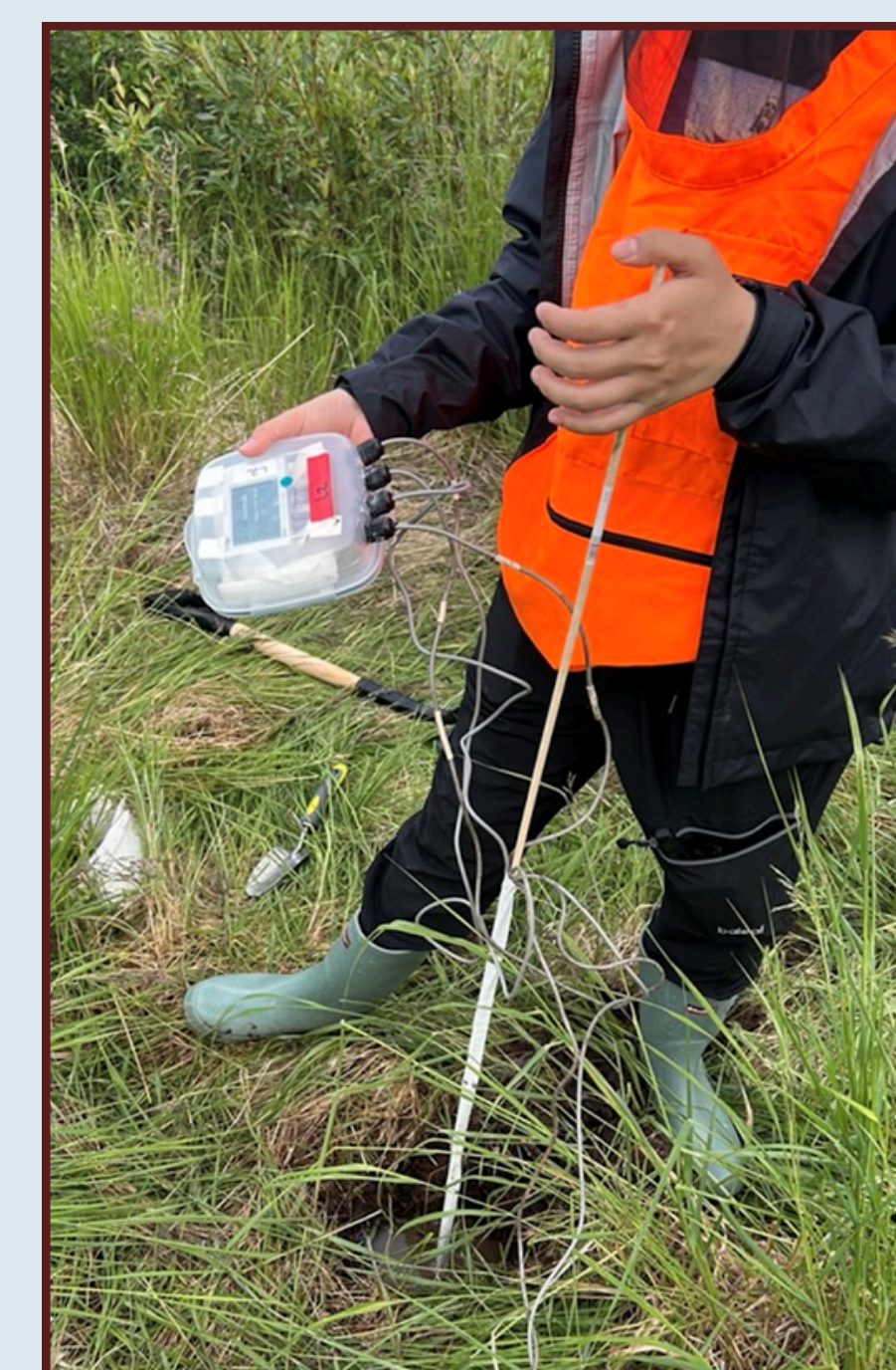
Figure 4: Photo of the Cryotic Assessment Temperature probe in the ground.
