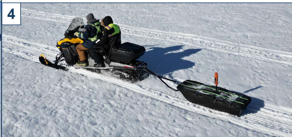
450 MHz ground penetrating radar (GPR) surveys were conducted along and across transects.
