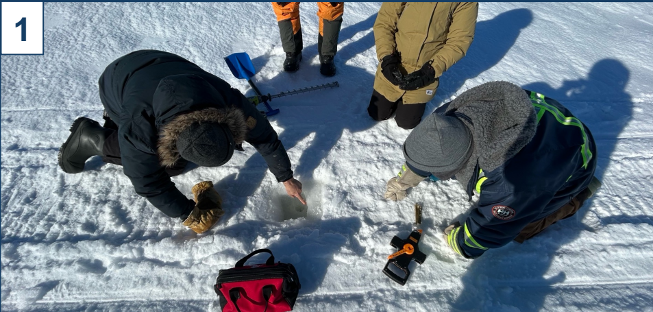
Snow and surficial ice layers were identified and measured using snow pits. Snow density samples were collected at certain snow pits.
