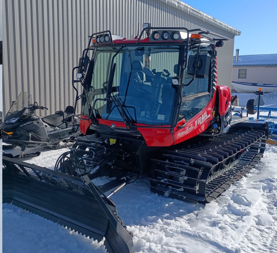
Conventional, mechanical groomer ~20,000 lbs fully-loaded
