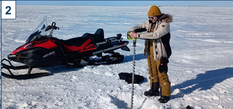
Ice thickness measurements were taken at the base of snow pits using a drill and weighted tape measure.
