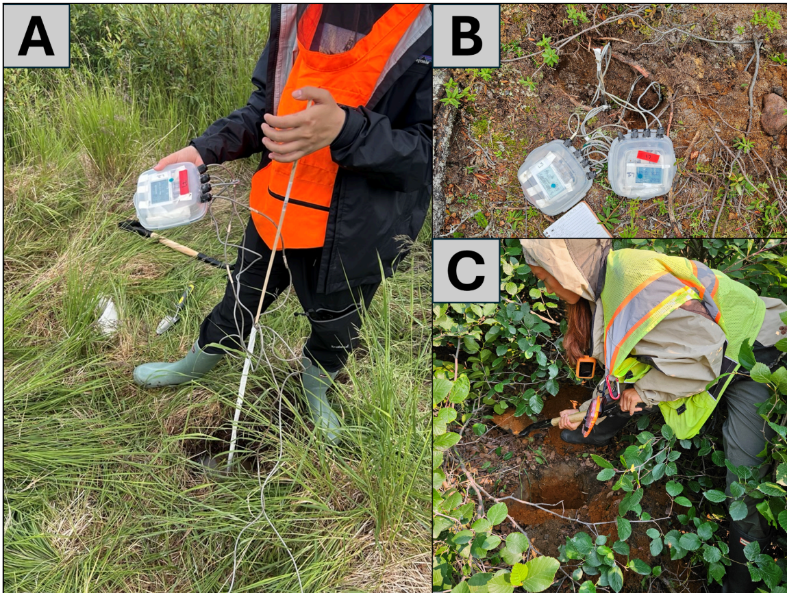
Figure 3.2: A) CAT probe in the ground; B) CAT probe and HOBO loggers in waterproof containers; C) Digging soil pit so frost probe can reach target depths.
